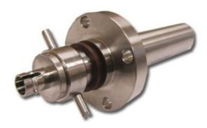
The FO310 is a sealed single-channel fiber optic rotary joint (FORJ) which is factory configured to transfer optical signals over either singlemode or multimode fiber. The FO310 supports both analog and digital optical signals, and is especially suited for sensitive single-pass optical sensing applications where optical insertion loss and back reflection must be minimized.
